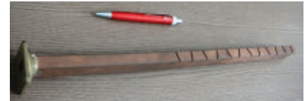
▲ Fig. 9 Slotted antenna made from a copper WR90 waveguide, top-milled by a CNC machine.
